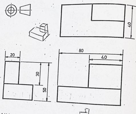
1.A Using the page provided complete both <u>Isometric</u> and <u>Oblique</u> simple sketches of the Cast Block.
